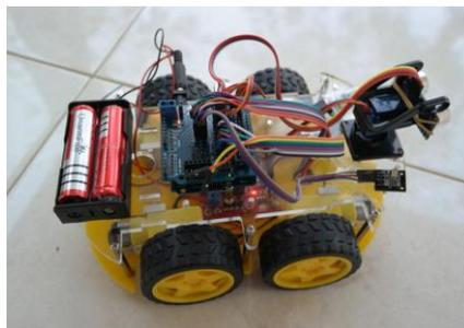
Gambar 5 Mobil remote control Arduino
